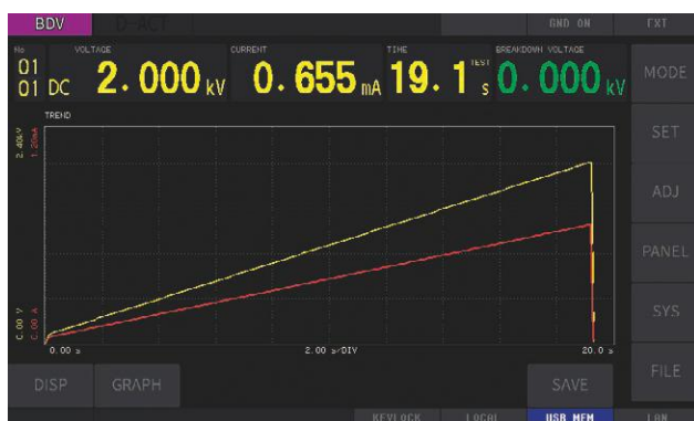
Example of continuous voltage rise test
