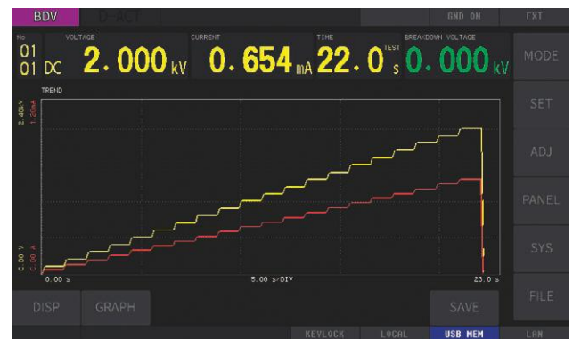
Example of stepped voltage rise testing
